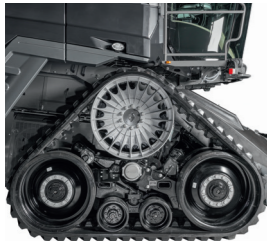
The TrakRide crawler drive minimises ground pressure.
