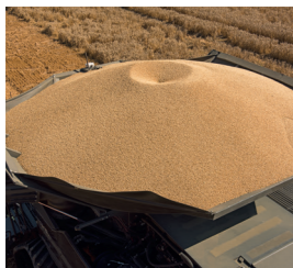
Volumes of up to 17,100 l in the Streamer 210 unload in around 81 seconds.
